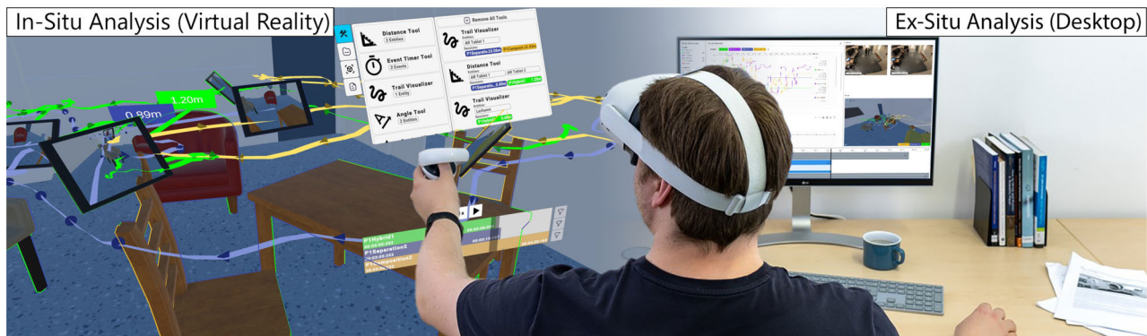
Figure 2: The ReLive mixed-immersion tool combines an immersive analytics virtual reality view (left) with a synchronized non-immersive visual analytics desktop view (right) for analyzing mixed reality studies. The virtual reality view allows users to relive and analyze prior studies in-situ, while the desktop facilitates an ex-situ analysis of aggregated data. [8].
