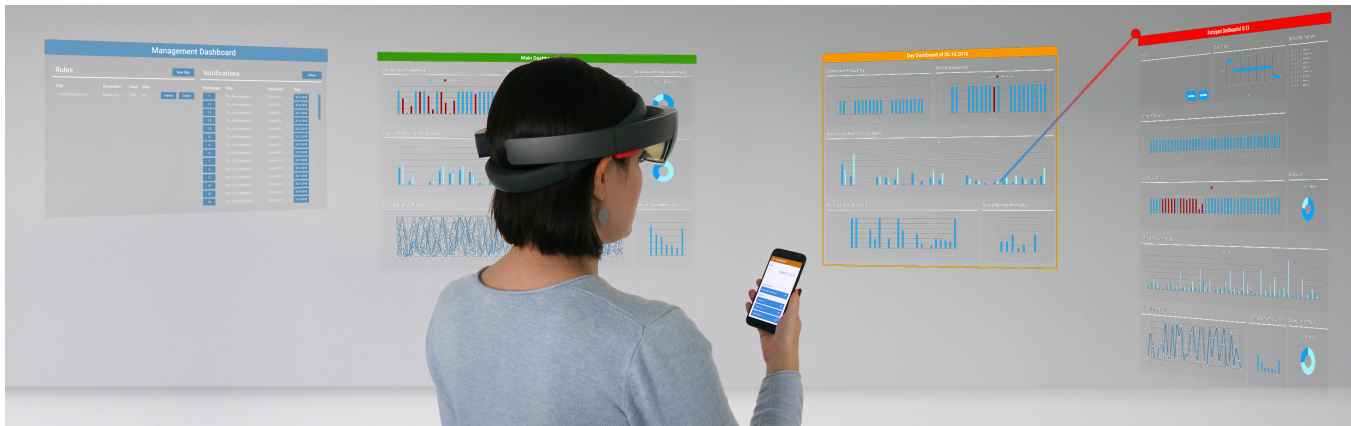
Figure 1: Interactive dashboards in augmented reality (IDIAR) visualize data from an ongoing mobile intervention study, enabling researchers to quickly identify irregularities. Four different dashboards provide users with both general and detailed information about an ongoing mobile intervention study. A multimodal interaction approach combining smartphone-based touch, head gaze, and voice input allows for familiar operation.
