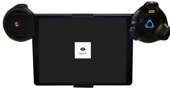
Figure 4.7: For the spatially-aware tablet, we attached Vive trackers to an iPad with the help of a custom 3D printed mount. Two trackers provide stable tracking, regardless of the tablet's orientation. The tablet's screen demonstrates the focus mode and thus only shows a single button to minimize distractions for the user.
