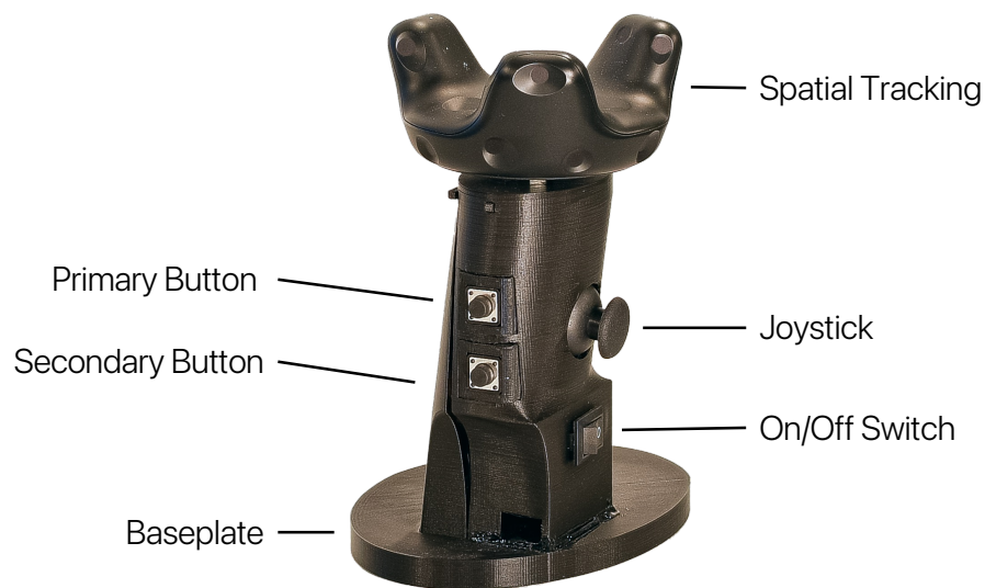
Figure 7.2: The SpatialMouse offers controls similar to a mouse and VR controller. The controls are mapped depending on the current mode: In mouse mode , the buttons are mapped to the left and right click, while the joystick acts as a mouse wheel replacement. In spatial mode , the buttons are mapped to the primary trigger and secondary button, while the joystick allows for 2D input. A spatial tracker at the top ensures consistent tracking in 3D space, while a baseplate on the bottom provides a wrist rest in mouse mode .
