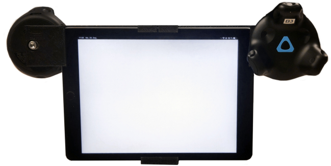
Figure 7: For the spatially-aware tablet, we attached Vive trackers to an iPad with the help of a custom 3D printed mount. Two trackers provide stable tracking, regardless of the tablet’s orientation.
