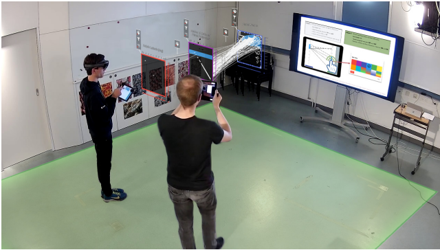
Figure 8: Our study setup provided users with ample space to move around (green, not visible during study). A large display was used to guide users through the first two tasks. The experimenter (right) could follow the participant’s progress in AR through the spectator viewer on a tablet.
