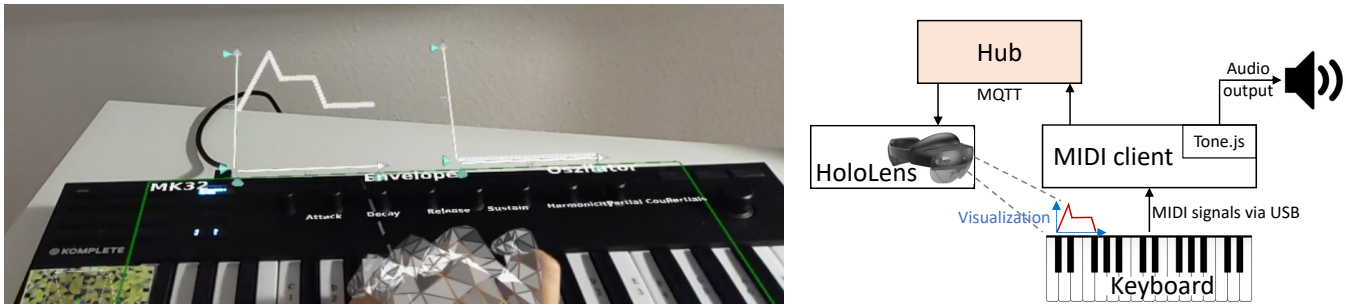
Fig. 15. (left) The ControllAR application overlays a visualization of the envelope curve on the corresponding inputs on the keyboard. (right) The responsibilities for this application are distributed across the keyboard (referent and physical input device), the MIDI client (responsible for sound synthesis and for converting MIDI events to MQTT events), the hub (here, only acting as a relay) and the AR client (compute envelope visualization and display it registered in the space above the keyboard).
